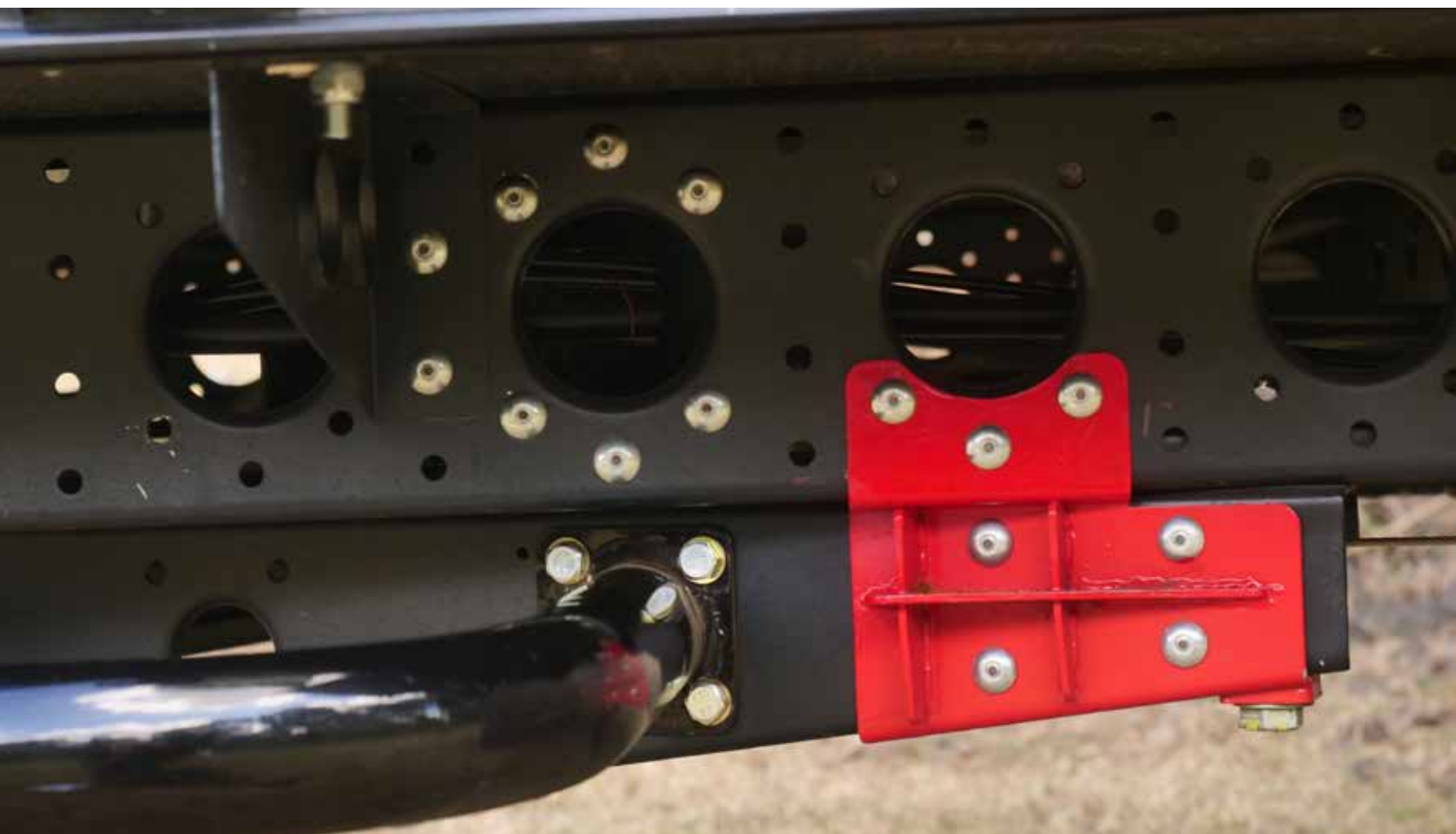
CLOCKWISE FROM ABOVE The chassis sections bolt and rivet together using punched profiles that save weight and add strength; The OTM 6.3 Adventure bristles with innovation and intelligent design; A very different-looking and practical storage box sits on the drawbar behind a Cruisemaster DO35 hitch
